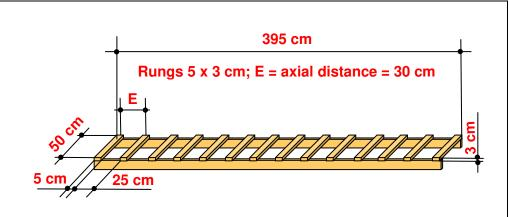
Beam ladder, length 4 m, rung distance 30 cm centered, rung width 5 cm, 14 rungs, 2 paddings at the start and end of the ladder: height approx. 0.50 m.
